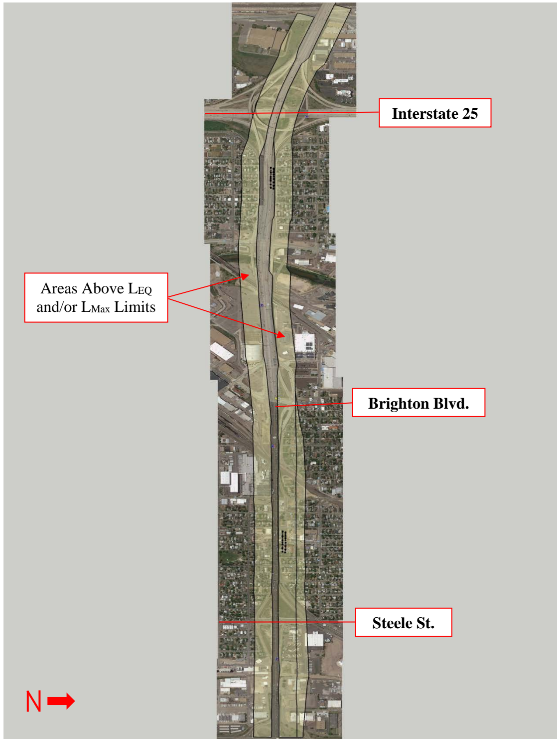
Figure 2: Construction Noise Extent for Excavation and Embankment Work
