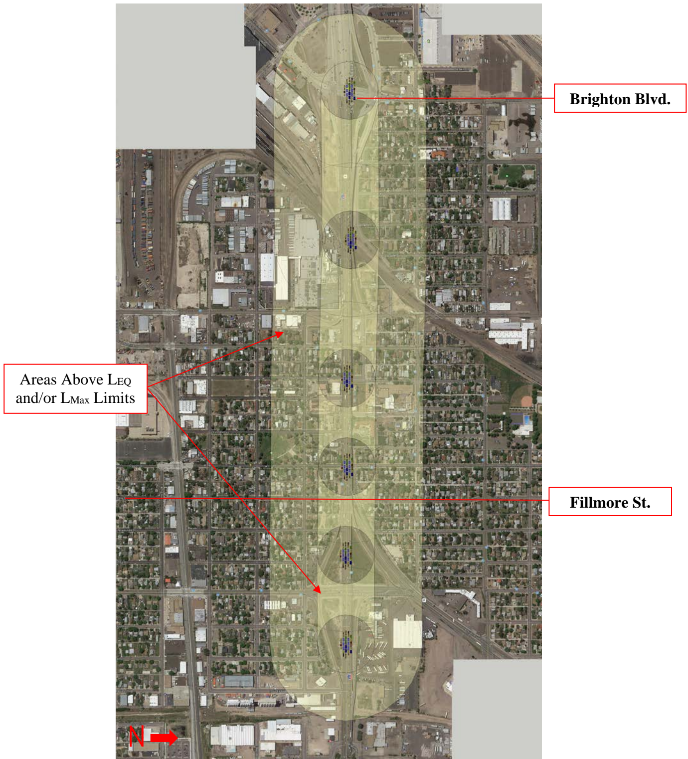
Figure 6: Bridge Demolition Noise L_{EQ} Distance/Radius
